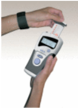
Figure 2: Oral Fluid NanoSensor Test (OFNASET) is a handheld, automated, and easy-to-use system that will be able to quickly and simultaneously detect multiple salivary protein and nucleic acid targets (Wong 2006).
